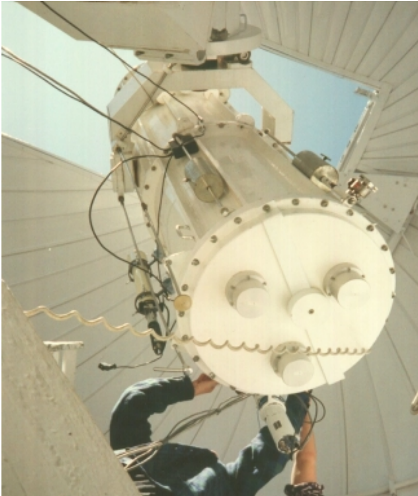
Figure 4: the 0.4m Vacuum Newtonian Telescope
