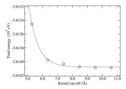
**Figure 1.** Convergence of the total energy of a Ti<sub>38</sub>O<sub>76</sub> cluster with respect to the density kernel cut-off
